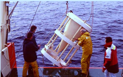
Deployment of a PPS5 Sediment trap (1 m 2 collecting area; carousel with 24 cups for sequential sampling) and schematic of the mooring line.
