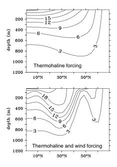
Figure 2: Upper-ocean temperature structure generated by an ocean general circulation and abiotic carbon-cycle model for an idealized ocean basin. The top panel shows the shallow diffusive thermocline that forms in the absence of wind forcing. The bottom panel depicts the solution with wind forcing in which the warm lens of the ventilated thermocline is evident in the subtropics.
